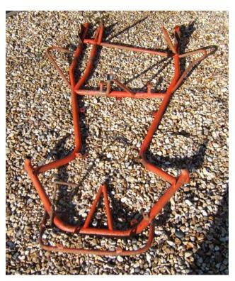
The bare chassis, with one pedal attached, because the front bar is bent the pedal would no come out. I checked dimensions diagonally and across the chassis and the main tubes seem ok, also the chassis sits flat (not just on gravel).
