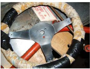
The wheel after an hour of wet and dry to get the surface smooth and another hour polishing with a mop and jewellers rouge followed by Autosol and black fingers. To protect the leather rim it was covered in period correct early 70's rag, attention to detail in the extreme. The two remaining gaiters were removed so I could clean them up and
