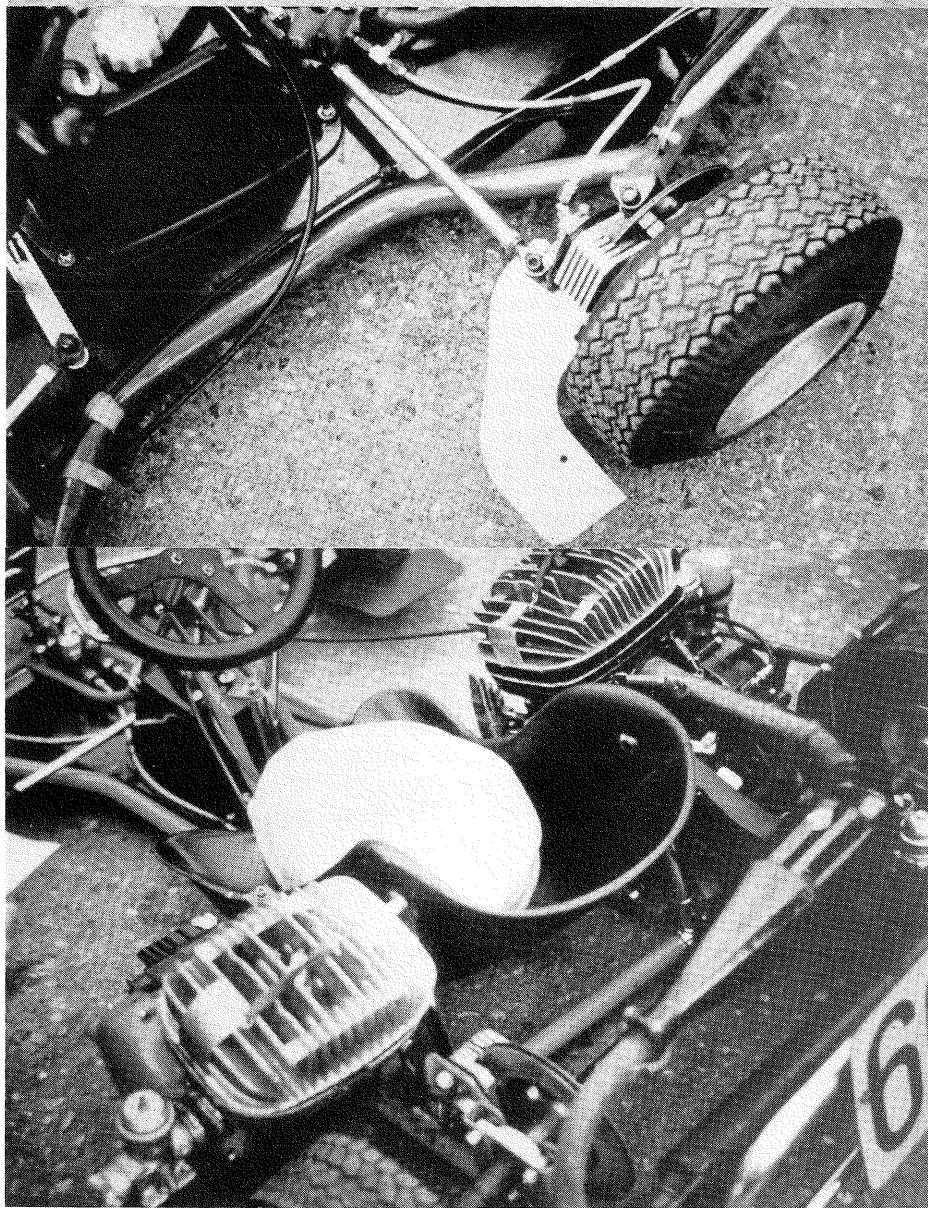
Top to bottom:- M. Ukbov of Moscow aboard the 125cc during the Parmi event. The outfit features a hand clutch and all round disc brakes are standard on the K-83 series, although from the picture it would seem only the rears are vented discs, and quite a novel idea for the steering mount, (probably seen better in the picture at the bottom left). Note also the brake pedal's twin mounting points. All karts feature centre tanks, but with the introduction of pods and bodywork this year, side tanks may well be introduced.
