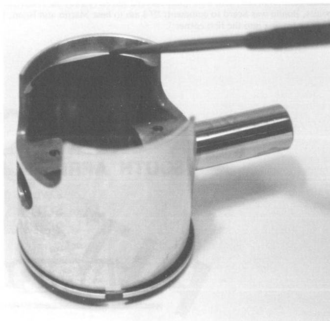
The edges indicated may be removed to prevent piston cracking.
