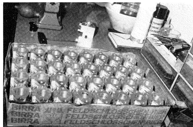
By necessity, the interior passages must be very accurate. This small drill set-up does the job.
